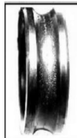
Figure 5.45 More obvious wear in the form of pits
