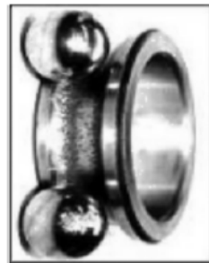
Figure 5.47 Severely damaged bearing in final stage of wear
